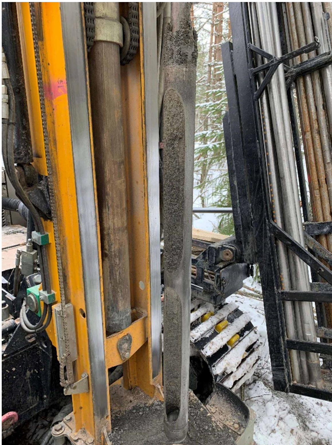
Figure 4. Drill rig and window sampler.
