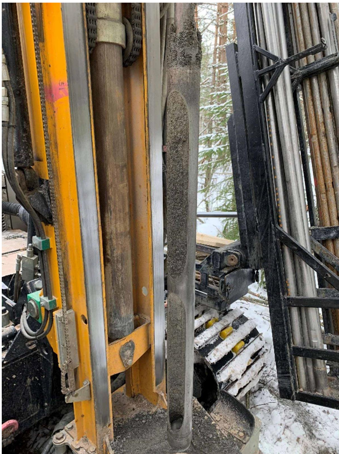
Figure 4. Drill rig and window sampler.
